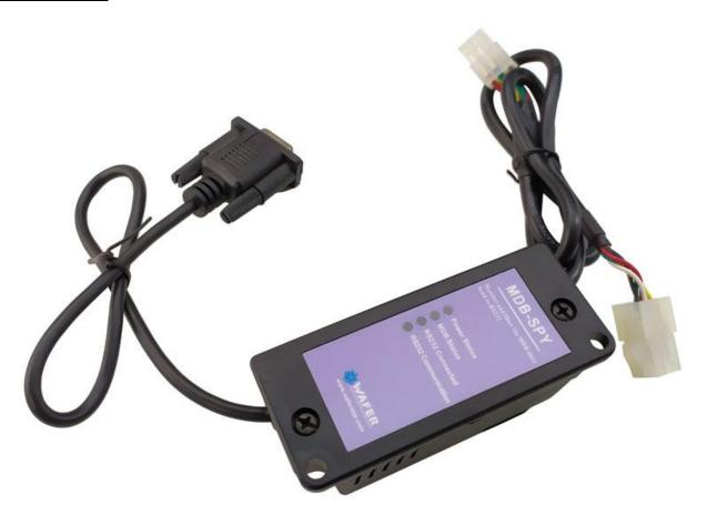
MDB-Spy Vending tools are an most useful tool for vending machine project engineers to develop or understand the MDB protocal and data.
